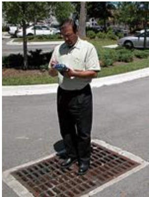
Using field software to collect information about a storm water structure.
